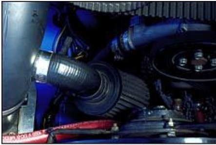
An airflow meter bypass will reduce injector pulse width and so can be used to compensate for larger injectors.
