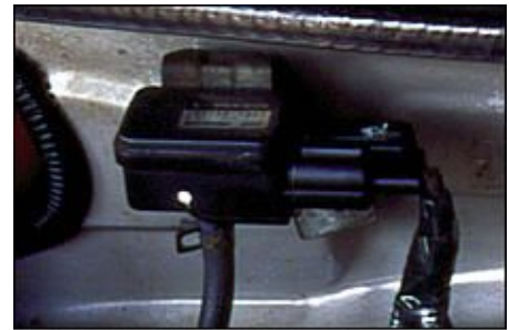
This car has had its MAP sensor output modified to run larger injectors. The wiring was done at the MAP sensor itself for ease of access.
