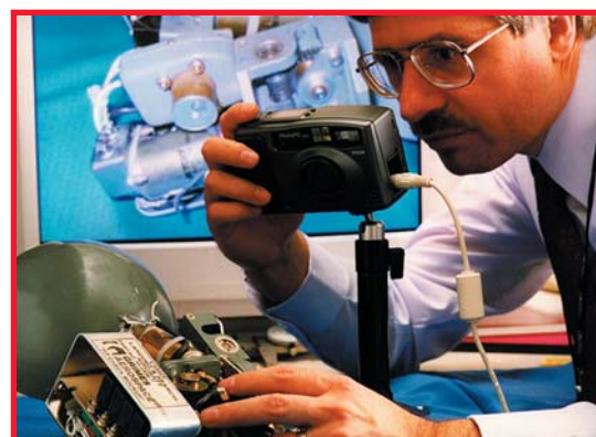
Using a digital camera, a Grimes technician records & stores the image of a problem helicopter search light on a PC. The image is then color plotted, printed or e-mailed for analysis. By examining repair trends, we can be proactive both in determining potential parts problems and in designing solutions.
