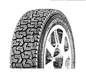
This tyre is suitable for use on loose, soft or gravel surfaces, generally offering low levels of grip. It is not recommended for applications on very abrasive surfaces. Its tread profile is flat with sharp edges, favouring directional stability and lateral grip; the blocks, arranged adially, guarantee excellent traction, particularly on loose ground.
